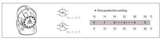
The required room temperature can be obtained by turning the handle of the thermostat unit.
