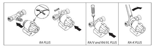
RA PLUS with snap-on coupling is easy to mount and requires no use of tools, once the valve cover has been removed.
