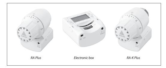
RA-PLUS is a programmable radiator thermostat that enables users to lower the individual room temperature by approx. 3° C during selected periods of the 24 hours of a day, thereby reducing heat consumption without any detrimental effects on comfort.
