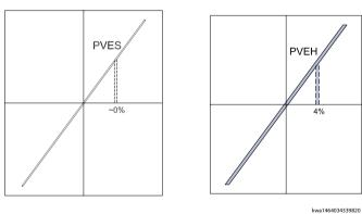
The PVES has an ASIC closed loop circuit and NC-S solenoids.
