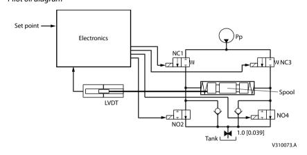
The hydraulic subsystem moves the spool and thereby opens the valve for work flow. The heart in the hydraulic subsystem is the solenoid valve bridge which controls the Pilot Pressure (Pp) on spool ends. It consist of four poppet valves, the two upper are normally closed (NC) and the two lower are normally open (NO).
