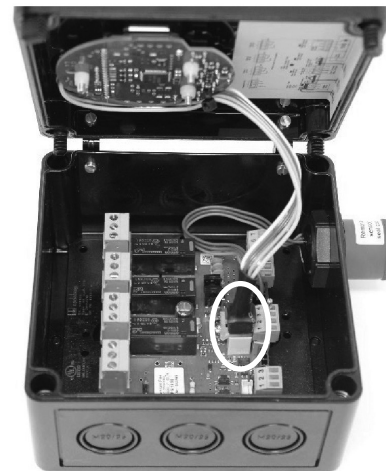
Figure 2: Unplug of the display PCB
