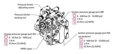
Endcaps are different for clockwise and counter clockwise rotation.
