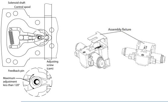
7. Pull assembly fixture out before installing control screws.
