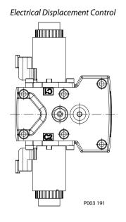
EDC schematic, feedback from swash plate
