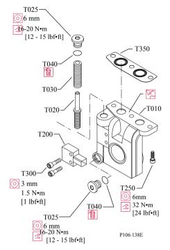
**1.** Remove three screws (T250) using a 6mm internal hex wrench.
