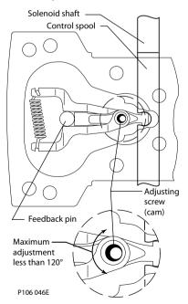
Illustration shows how cam on adjusting pin rotates to adjust for neutral position after pump is reinstalled.
