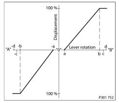
Deadband on **B** side:  $\mathbf{a} = \mathbf{3}^{\circ} \pm \mathbf{1}^{\circ}$ Maximum pump stroke:  $\mathbf{b} = \mathbf{30}^{\circ} + 2/-1^{\circ}$ Required customer end stop:  $\mathbf{c} = \mathbf{36}^{\circ} \pm \mathbf{3}^{\circ}$ Internal end stop:  $\mathbf{d} = \mathbf{40}^{\circ}$
