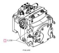
1. To open the HPRVs (L150), rotate three revolutions counterclockwise using a hex wrench.
