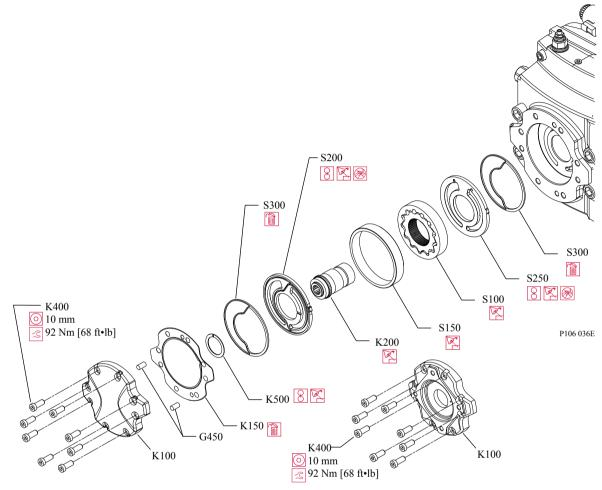
1. Using a 10 mm internal hex wrench, remove cap screws (K400).
