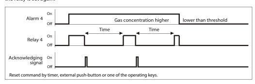
5.7.2.6 External Override of Alarm / Signal Relay via DI
