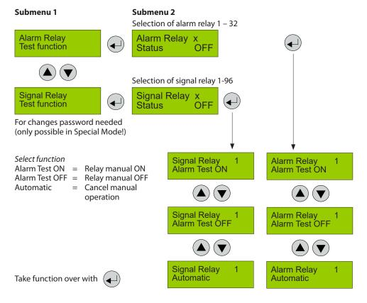
The test function sets the target device (selected relay) in Special Mode and activates a timer that reestablishes the normal measurement mode after 15 minutes and ends the test function.
