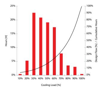
As can be seen from the graph above, full load is not common in HVAC systems. Several reasons for this can be identified:
