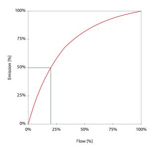
The coil characteristic is quite aggessive. So, 50% of the maximum output can be achieved with only 20% of the flow.
