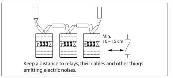
When controllers are fitted in a cabinet door, the cables are usually kept together in bundles of cables. Here the bundle with data communication, display and digital input signals must be kept separate from other cables that emit noise.
