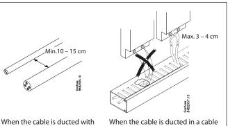
When the cable is ducted with other cables, there is a strong risk that electrical noise will be transferred. Keep away from live cables. When the cable is ducted in a cable tray, the **cable** must be fed out and right up to the controller. The fast solution where only wires are fed out will cause problems.
