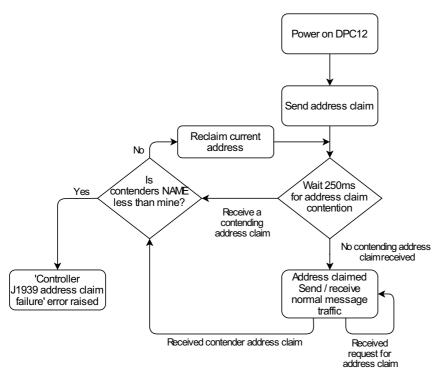
For the full address claim procedure refer to SAE J1939 standard or contact your Danfoss representative.
