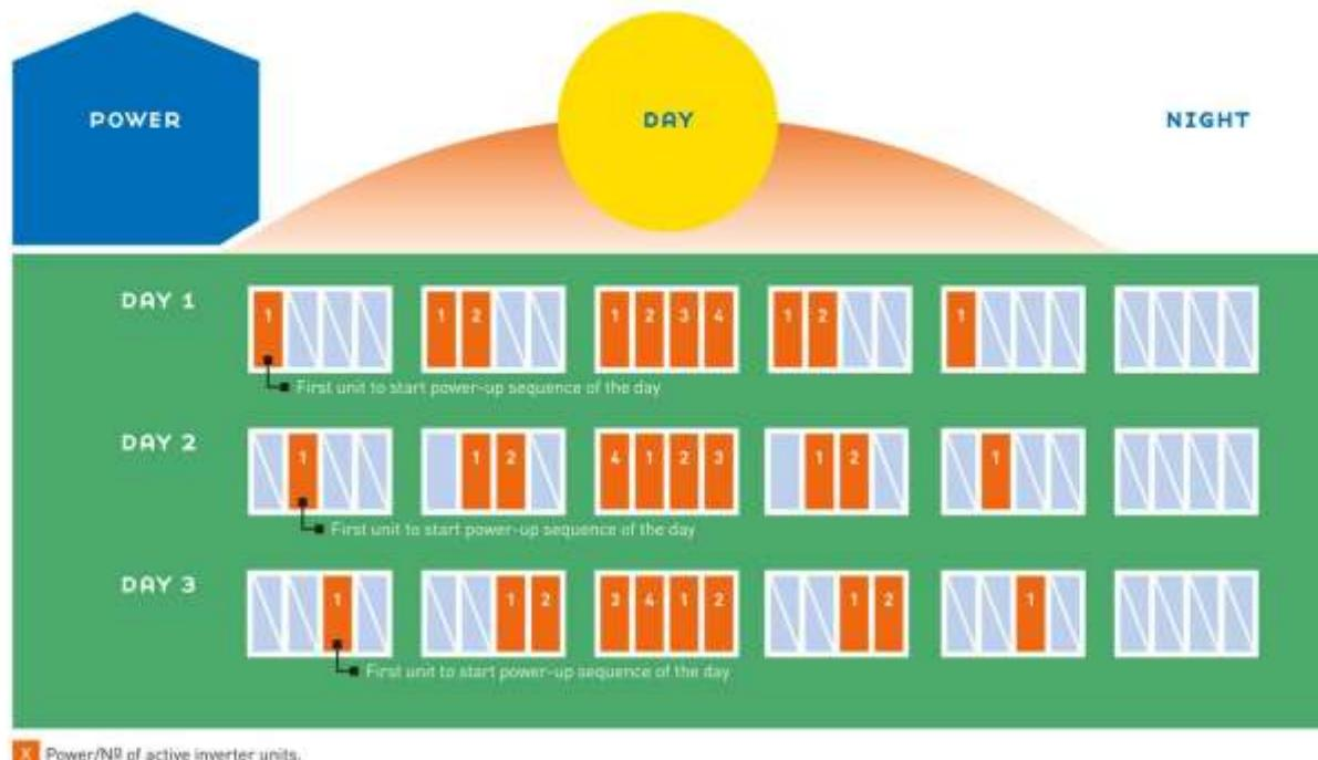
*Picture 2. Multi master system master change function.*
