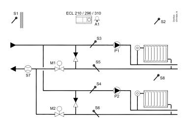
Weather compensated control of flow temperature in two heating circuits. Room temperature compensation and sliding return temperature limitation. Circuits independent in parallel or circuit 2 after circuit 1.
