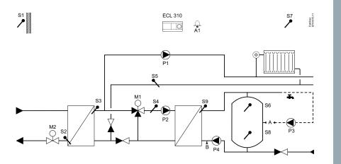
Weather compensated control of flow temperature in heating circuit. Room temperature compensation and sliding return temperature limitation.
