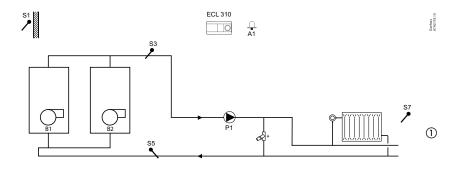
Weather compensated flow temperature control of 1-stage boiler based heating systems. One direct heating circuit and one mixing circuit. Circulation pumps control, room temperature control and sliding return temperature limitation.
