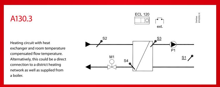
Flow temperature based on compensated supply temperature (offset).
