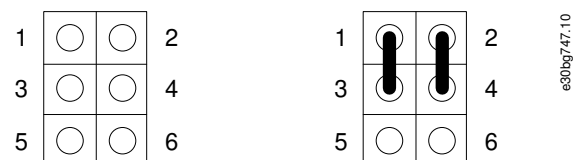
Illustration 88: Jumper Pin Sequence and Connection Example (Pins 1-3 and 2-4 Connected)
