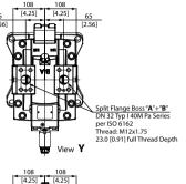
Split Flange Boss "**A**" + "**B**" DN 32 Typ I 40M Pa Series per ISO 6162 Thread: M12x1.75 23.0 [0.91] full Thread Depth
