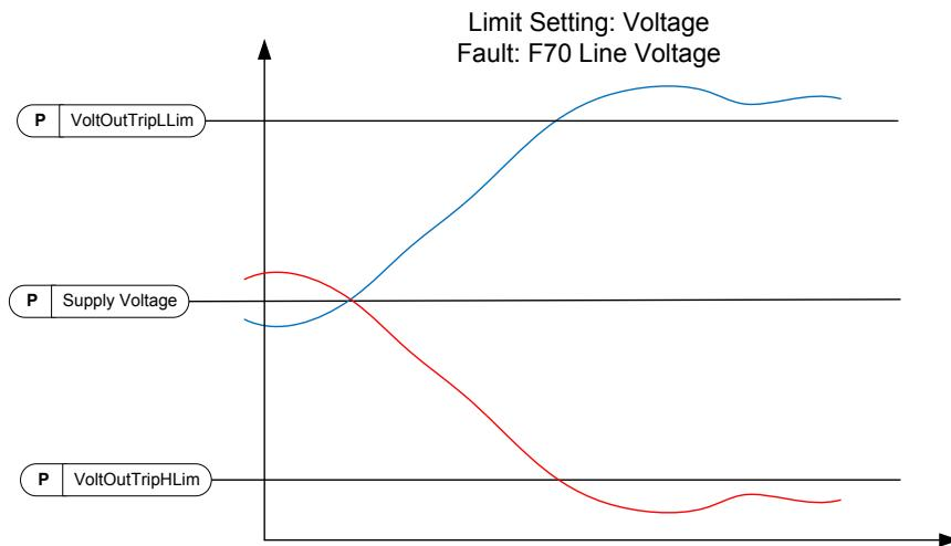
Note: This monitor voltage at drive terminal. When compensating LCL terminal voltage, Output voltage may be considerably higher on full load situations than given Supply Voltage
