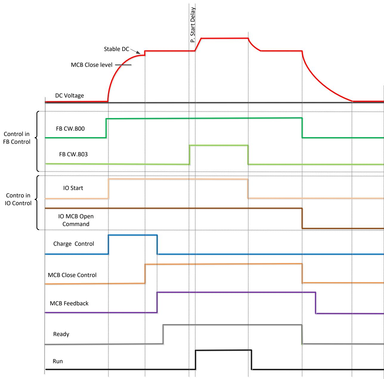
Above example when "Standard" state machine is used. With "Basic" state machine operation is like in IO Control.
