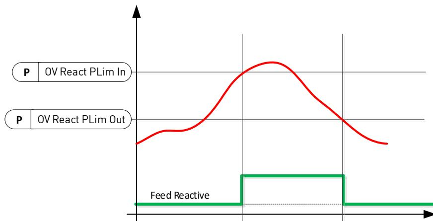
7.16.6.3 Power Lock In and Out Reference under voltage.
