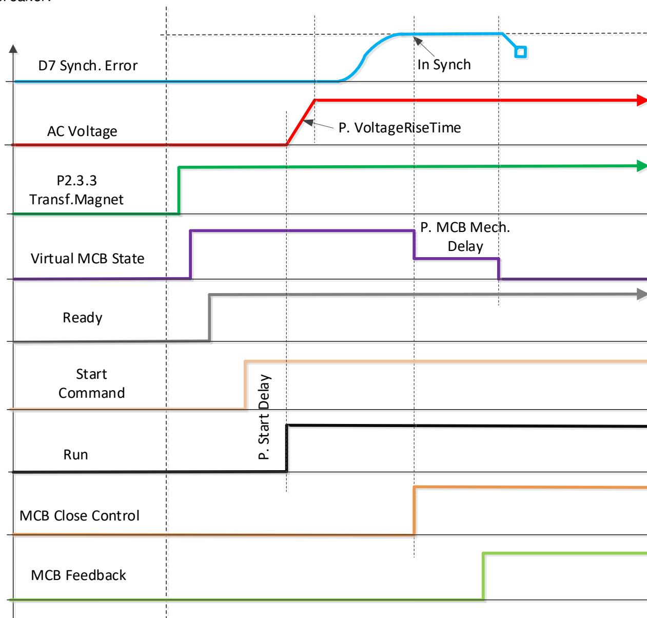
MCB breaker mechanical delay can be compensated with P2.5.7.7 MCB Mech. Delay ID1967
