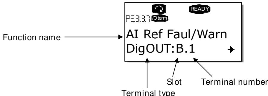
**Example:** You want to connect the digital output function Reference fault/warning (parameter 2.3.3.7) to the digital output DO1 on the basic board NXOPTA1 (see VACON® NX User Manual).
