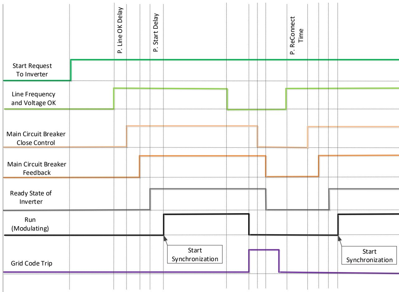
Note: Drive needs to see grid within OK limits for voltage and frequency before MCB is closed and drive started.
