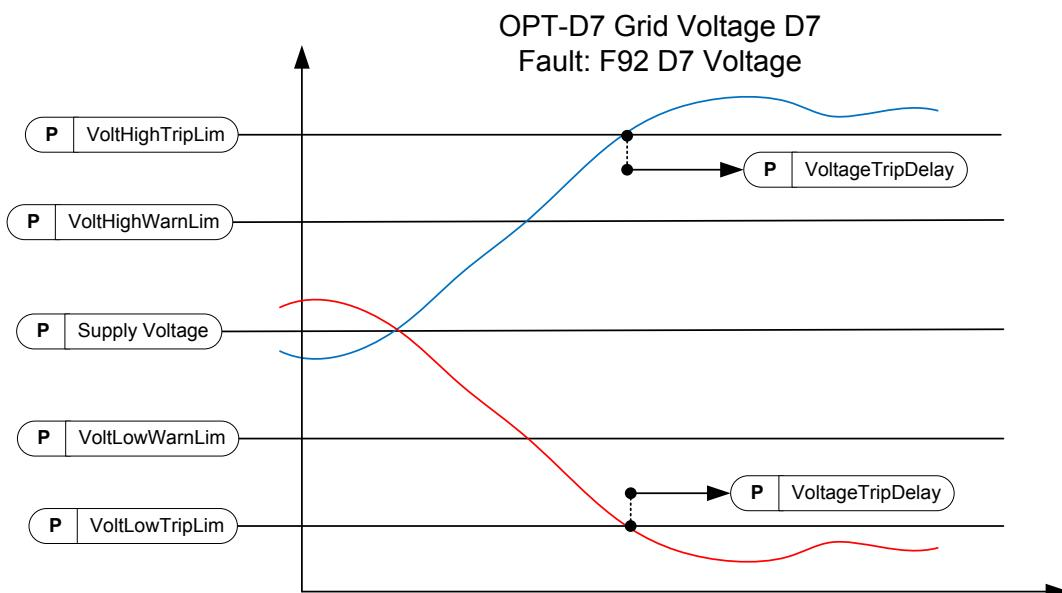
Note: Low Voltage trip from D7 board is disabled if drive has detected Short Circuit
