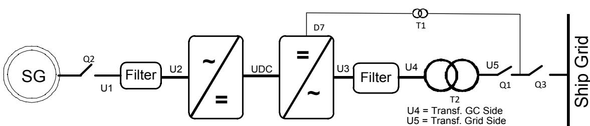
First Voltage Droop and Frequency Droop are set to the same values as the diesel generators on the ship's grid.
