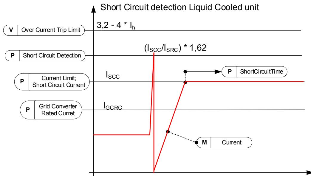
In this case Short Circuit Level 264% would be equal to Current Limit in rms. The recommended value for the Short Circuit Level in the case above is 304 %. The function will be disabled if a value above 499% is given.
