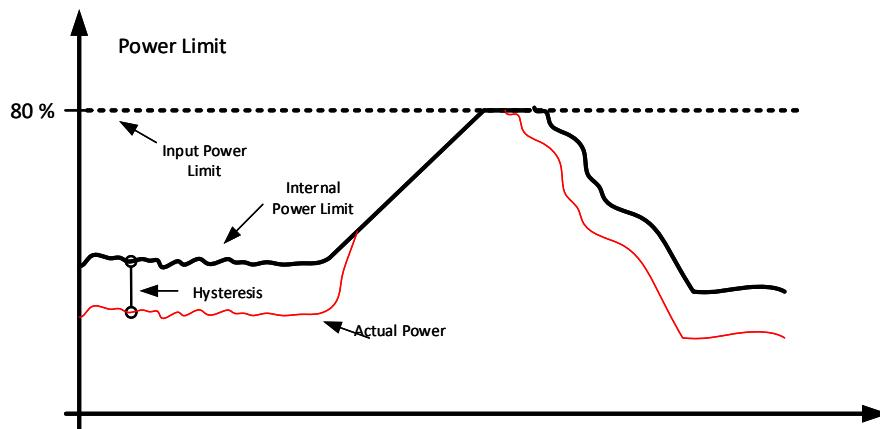
**P2.17.11.2 Maximum Output Power with Grid Codes** **ID3397** **"GC Max Power"**
