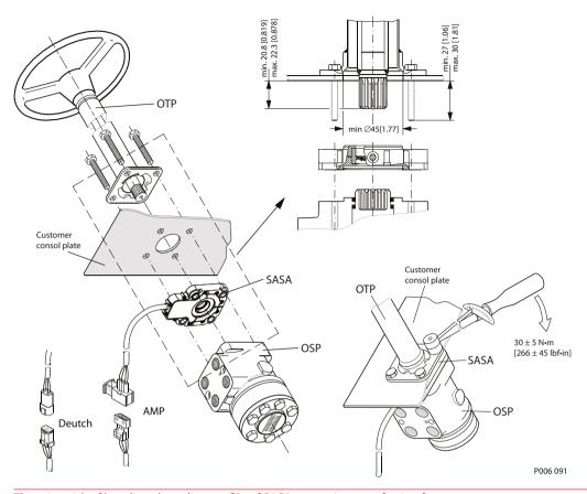
There is a risk of bending the spline profile of SASA sensor in case of using force.
