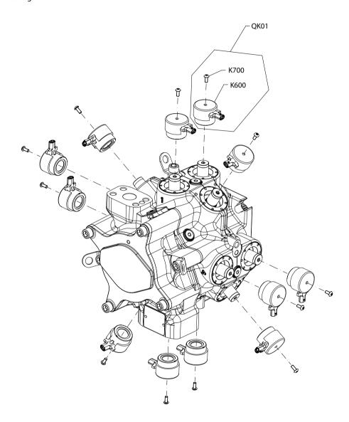
Generic housing (single-outlet pump) and valve coil cores used to show part location only.
