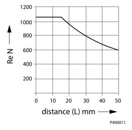
Danfoss recommends clamp-type couplings for applications with radial shaft loads
