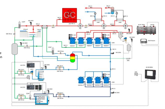
High pressure (50-120 bar) Receiver pressure (32-50 bar) MT suction pressure (22-36 bar) LT suction pressure (10-16 bar)
