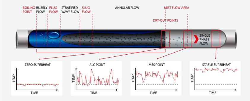
Danfoss Adaptive Minimum Stable Superheat Control (MSS)
