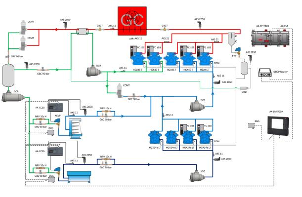
High pressure (50-120 bar) Receiver pressure (32-50 bar) MT suction pressure (22-36 bar)
