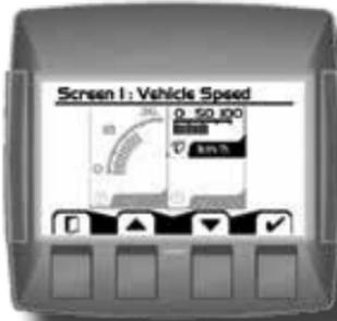
**4.** After making a signal selection, press the right arrow (Next) soft key to go to the next selection area. Use the up, down arrow, next and select soft keys to select signal. Select the right arrow soft key to move to the next selection area.
