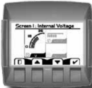
**3.** After screen type selection, select signals to monitor. Use the up and down arrow soft keys to cycle through available signal selections.
