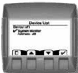
The Device List page will list all J1939 devices and addresses that are currently being monitored on the network.
