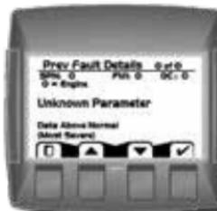
Selecting Previous Faults in the Fault Menu will display all previously active faults on the CAN network.
