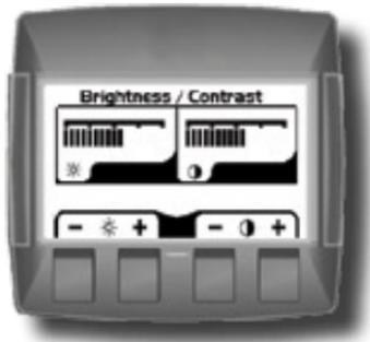
Adjust brightness and contrast levels by pressing soft key 2. This will display the brightness and contrast soft key bar. The bar will disappear after 3 seconds of inactivity.
