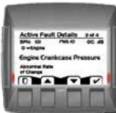
Selecting Active Faults in the Fault Menu will display all active faults on the CAN network.
