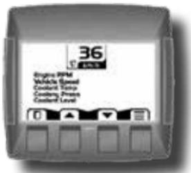
The Quick Data function allows selected signals to be monitored in a scrollable single view display.
