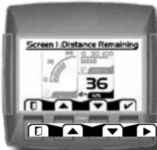
**5.** Using the right arrow soft key will rotate through the selections in a clockwise rotation.
