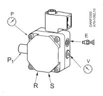
Note! Shaft rotation, location of nozzle outlet and other connections are seen from shaft end.
