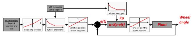
The algorithm can be broken down and explained in five parts:
