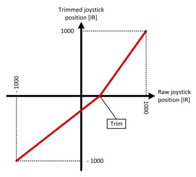
The example above shows a situation where the joystick neutral position has been trimmed to the right.
