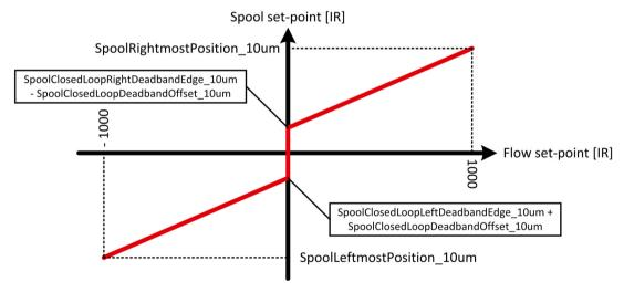
For optimal closed loop joystick steering performance, it is important that the spool calibration parameters are correct.
