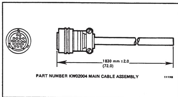
FIGURE 6. Main Cable Assembly.
