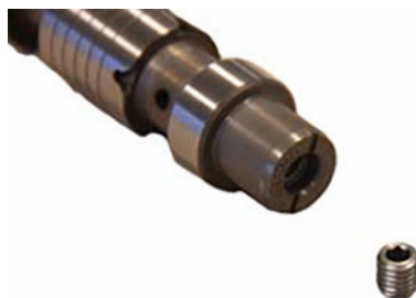
Dismantled directional spool (25) and orifice (26)
