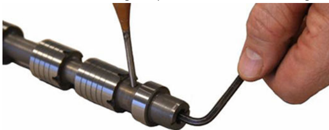
Dismantled directional spool (25) and orifice (26)
