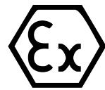
[2] **Equipment or Protective Systems or Components intended for use in Potentially Explosive Atmospheres**
