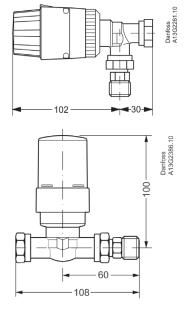
Add 32 mm to allow for sensor removal/fitting
