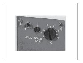
The ETS is a stand alone snow melt controller that provides an economical method for removing the accumulation of snow or ice in unwanted areas.
