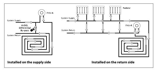
The water supply temperature for the system should be properly monitored to ensure the surface temperature is appropriate for the finished floor material.
