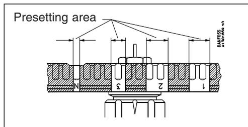
The presetting can be set at the values: 1- 2 - 3 and N. At setting N, the valve is completely open. A setting in the shaded areas should be avoided. When the sensor element is mounted, the presetting is hidden, and is thus protected against alteration.
