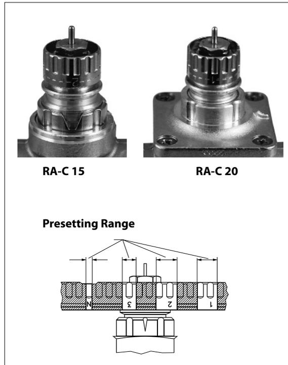
The incorporated pre-settable option on the RA-C valve body has an easy setting adjustment ring with clearly engraved setting markers scaled 1-2-3 and N, with N being the completely open position. Setting the appropriate value is quick and precise, without the need for a special tool. A setting in the shaded areas should be avoided. Refer to Capacity charts for proper pre-setting values. To pre-set the valve:
