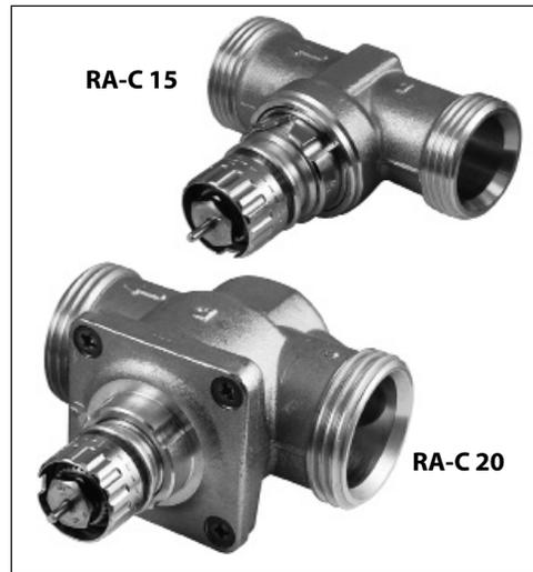
RA-C is a high capacity two-port valve used in the regulation of hot or chilled water in hydronic systems. The RA-C's actuator mounting connection is identical to the RA2000 family, allowing a wide selection of thermostatic & electric actuators to suit hydronic applications such as chilled ceilings, chilled beams, fan coils & induction units for heating/cooling, & radiators.
