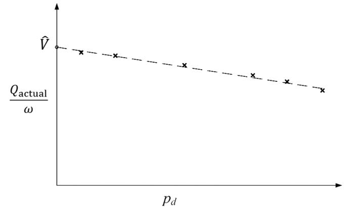
Figure 5: Zero-pressure intercept method for derived displacement volume
