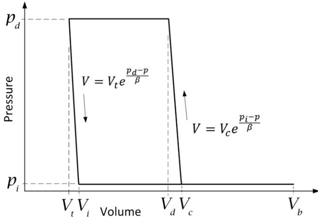
Figure 2: Pressure-volume diagram for a single piston,  $x = 0.5$
