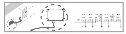
**4.** Check if the electrical installation and verify if there's an option to connect the neutral or the ground cable. In that case, don't forget to connect the ground cable.
