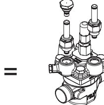
ICV 32 valve body w/different connections      Table I
