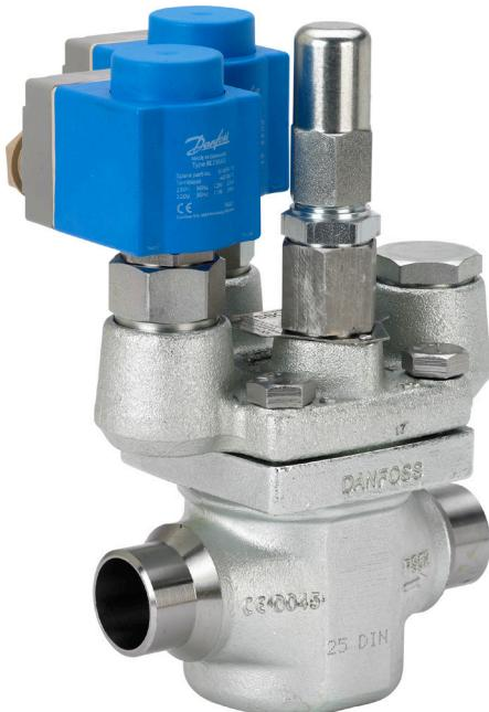
ICSH dual position solenoid valve belongs to the ICV family and consists of an ICV housing, an ICS insert together with an ICSH top cover with 2 EVM normally closed solenoid pilots installed in the top cover.
