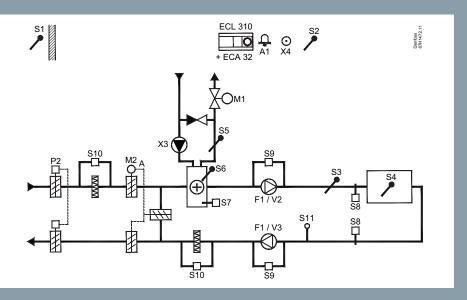
Advanced temperature control of DHW circuit with storage tank, directly heated or charging system. Return temperature limitation. Optional temperature control of DHW heating temperature.
