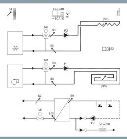
Weather compensated flow temperature control of heating / cooling circuit(s). Automatic change-over between heating and cooling. Circulation pump control. Dew point (cooling mode only) and surface temperature compensation. Return temperature limitation.
