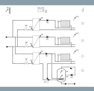
Subtypes A390.3, A390.11, A390.12 and A390.13 have for the control valve 3-point outputs as well as 0 – 10 V outputs
