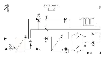
Weather compensated control of flow temperature in heating circuit. Room temperature compensation and sliding return temperature limitation.
