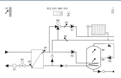
Weather compensated control of flow temperature in heating circuit. Room temperature compensation and sliding return temperature limitation.
