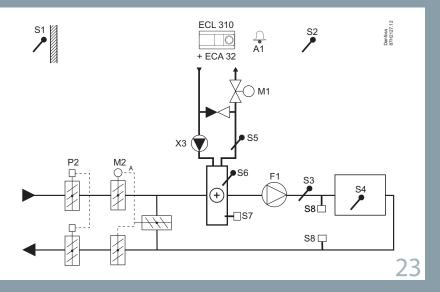
Multi purpose application. Temperature control of, for example, ventilation systems with heating or cooling or a combination of these. Weather based compensation, return temperature limitation, frost and fire protection. Optional analog control of cross-flow or rotary heat exchanger.
