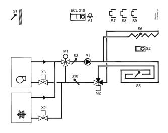
Weather compensated control of flow temperature in heating circuit. Room temperature compensation and sliding return temperature limitation.
