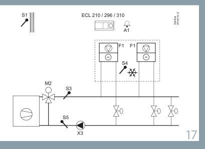
Multi purpose application. Temperature control of, for example, ventilation systems with heating or cooling or a combination of these. Weather based compensation, return temperature limitation, frost and fire protection. Optional analog control of cross-flow or rotary heat exchanger.
