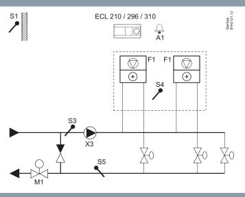
Multi purpose application. Temperature control of, for example, ventilation systems with heating or cooling or a combination of these. Weather based compensation, return temperature limitation, frost and fire protection. Optional analog control of cross-flow or rotary heat exchanger.
