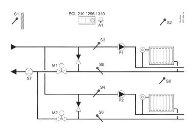
Weather compensated control of flow temperature in two heating circuits. Room temperature compensation and sliding return temperature limitation. Circuits independent in parallel or circuit 2 after circuit 1. Alarm function related to flow temperatures.
