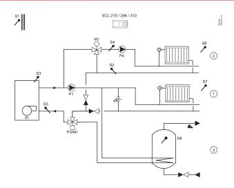
Weather compensated flow temperature control of 1-stage boiler based heating systems. One direct heating circuit and one mixing circuit. Circulation pumps control, room temperature control and sliding return temperature limitation.
