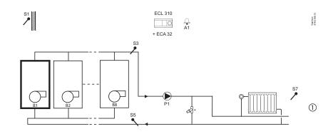
Weather compensated flow temperature control of 1-stage boiler based heating systems. One direct heating circuit and one mixing circuit. Circulation pumps control, room temperature control and sliding return temperature limitation.
