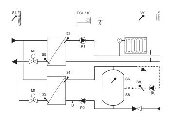
Weather compensated control of flow temperature in two heating circuits. Room temperature compensation and sliding return temperature limitation. Circuits independent in parallel or circuit 2 after circuit 1.
