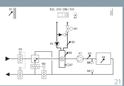
Multi purpose application. Temperature control of, for example, ventilation systems with heating or cooling or a combination of these. Weather based compensation, return temperature limitation, frost and fire protection. Optional analog control of cross-flow or rotary heat exchanger.
