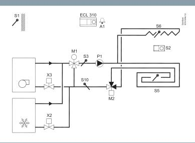
Weather compensated flow temperature control of heating / cooling circuit(s). Automatic change-over between heating and cooling. Circulation pump control. Dew point (cooling mode only) and surface temperature compensation. Return temperature limitation.
