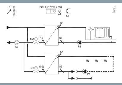
Weather compensated flow temperature control of 1-stage boiler based heating systems. One direct heating circuit and one mixing circuit. Circulation pumps control, room temperature control and sliding return temperature limitation.
