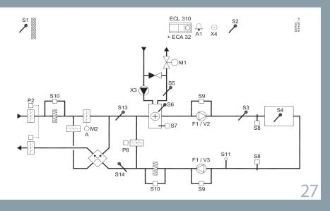
Multi purpose application. Temperature control of, for example, ventilation systems with heating or cooling or a combination of these. Weather based compensation, return temperature limitation, frost and fire protection. Optional analog control of cross-flow or rotary heat exchanger.
