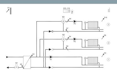
Subtypes A390.3, A390.11, A390.12 and A390.13 have for the control valve 3-point outputs as well as 0 – 10 V outputs.
