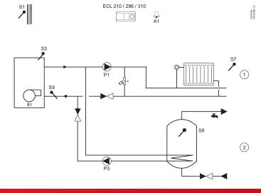
Weather compensated flow temperature control of 1-stage boiler based heating systems. One direct heating circuit and one mixing circuit. Circulation pumps control, room temperature control and sliding return temperature limitation.
