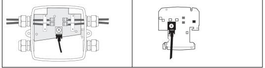
3. Turn the transmitter connection board so that the connection cable is facing downwards.
