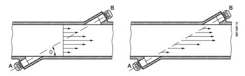
Figure 3-1 Velocity distribution along sound path
