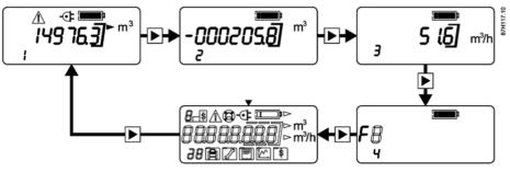
Figure 6-1 Operating the local display
