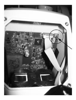
Figure 7-3 HW key behind the display (placed on the right pins)
