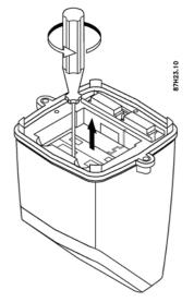
2. Fit new battery pack in transmitter.
