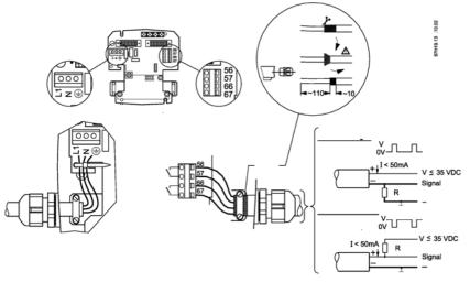
Figure 5-2 Output and power supply connection
