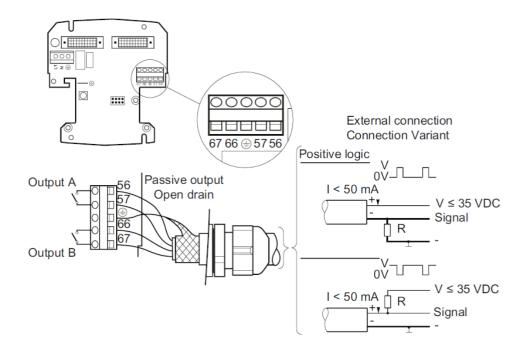
4. Tighten cable gland for output cable(s) (approx. 20 Nm).
