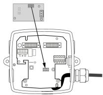
3. Fasten module to transmitter connection board by use of a M3x5 screw (0.5 Nm).
