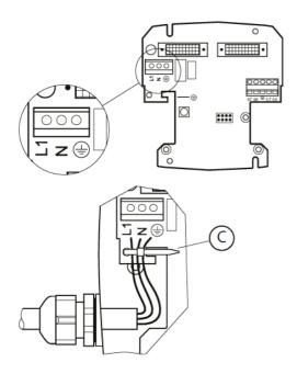
5. Tighten cable gland for power supply cable (approx. 20 Nm).
