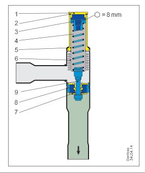
Crankcase pressure regulator type KVL opens on a fall in pressure on the outlet side, i.e. when the suction pressure falls below the set value.
