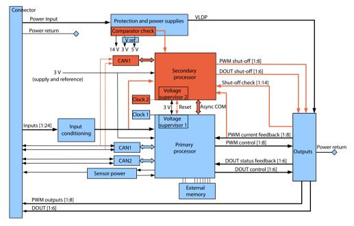
The PLUS+1 $^{\circ}$  SC0XX-1XX Controller is classified as a Type B $^{1}$  high demand mode component with HFT = 0 per IEC 61508.
