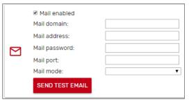
The device can be configured to send a notification via email when the status of the application alarm changes.
