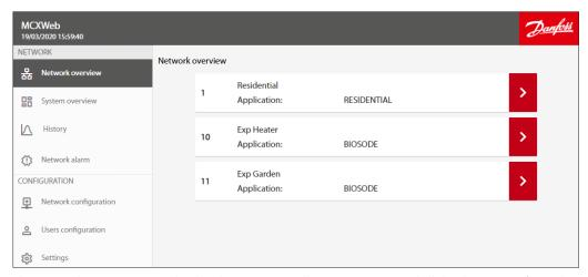
The Network overview is used to list the main controller MCX15/20B2 and all the devices configured in the Network Configuration and connected to the main controller through fieldbus (CANbus). For each configured MCX the following information is displayed:
