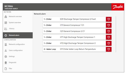
This page shows the list of the alarms active for **all** the devices connected to the fieldbus (CANbus). Alarms for each individual device are also available on the device pages.
