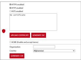
Enable HTTPS with personalized server certificate if the device is not in a secure environment. Enable HTTP if the device is in a secure LAN with authorized access available (also VPN). Enable HSTS if you want to force web browsers to interact with the device only via secure HTTPS connections (and never HTTP). This helps to prevent protocol downgrade attacks.
