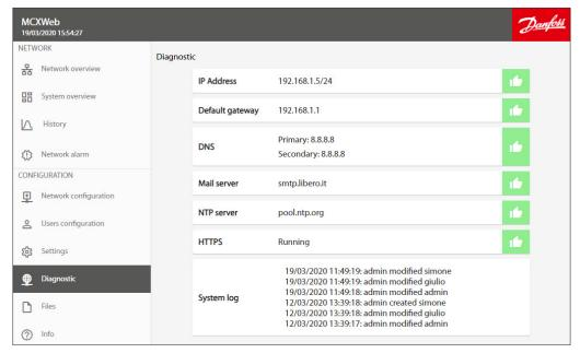
This section is useful for verifying your network configuration and seeing which protocols are active and whether the corresponding destinations are reachable, if relevant. In addition, a *System log* is displayed where events of major importance concerning security are recorded.
