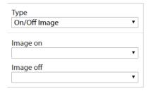
the *Image on* and *Image off* fields can be used to associate different images to the ON and OFF value of a Boolean variable. A typical usage is to have different icons for the alarm ON and OFF states. The On/Off images must have been loaded previously through the *Files* menu (see *3.4 Files*).
