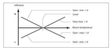
This limitation is based on a PI regulation where P (Gain) responds quickly to deviations and I (Intgr. time) responds slower and over time removes the small offsets between the desired and actual values. This is done by changing the desired flow temperature.
