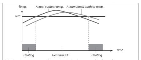
This function can save energy by stopping the heating system when the outdoor temperature gets above a set limit. The heating system switches ON again when the outdoor temperature and the accumulated outdoor temperature become lower than the set limit.
