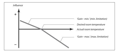
Set a positive value for the 'Gain - min.' and a negative value for the 'Gain - max.'.
