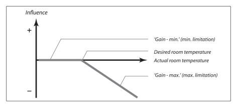
The 'Gain - max.' determines how much the room temperature should influence the desired flow temperature.
