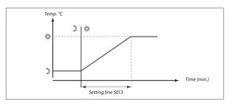
In order to avoid load peaks in the supply network, the flow temperature can be set to increase gradually after a period with setback temperature. This causes the valve to open gradually.
