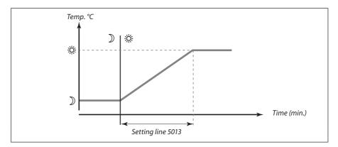
In order to avoid load peaks in the supply network, the flow temperature can be set to increase gradually after a period with setback temperature. This causes the valve to open gradually.
