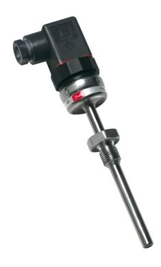
With MBT 3560 we have combined the technology of our standard temperature sensors and the electrical connections from our MBS pressure transmitters with a new developed electronics which has resulted in a compact temperature sensor with a built-in transmitter.
