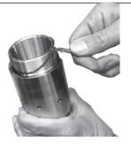
2. Remove the O-ring at the thread end of the valve with a small screw driver.
