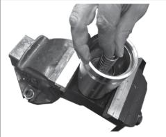
5. Mount the spring on the rod of the cone.
