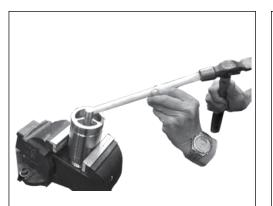
3. Alternatively use a mandrel made of nylon.
