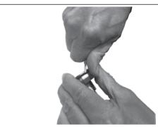
7. Remove the O-ring at the cone with a small screw driver.
