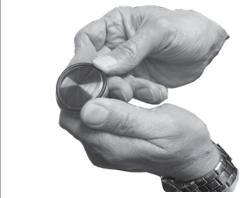
3. Mount the water lubricated O-ring on the cone. Ensure the O-ring is pushed fully into the O-ring groove.
