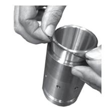
2. Mount the lubricated O-ring at the thread end of the valve.
