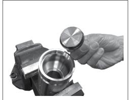
6. Remove the valve cone.
