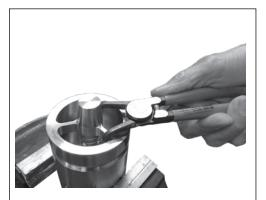
2. Turn the nut CCW with snap ring pliers.
