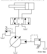
The remote PC control uses a pilot line connected to an external hydraulic valve. The external valve changes pressure in the pilot line, causing the PC control to operate at a lower pressure. When the pilot line is vented to reservoir, the pump maintains pressure at the load sense setting.
