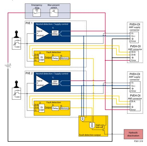
Fault monitoring for deactivation of the hydraulic system with extra fault inputs using the PVE's with DI (Direction Indication) function. System Control Logic, example PLUS+1® for signal monitoring and triggering signal for deactivation of the hydraulic system.
