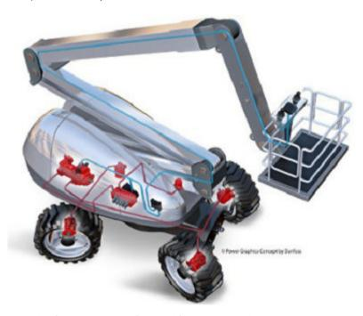
Example of a control system for man-lift using PVE Fault monitoring input signals and signals from external sensors to ensure the PLUS+1° main controllers correct function of the man-lift.
