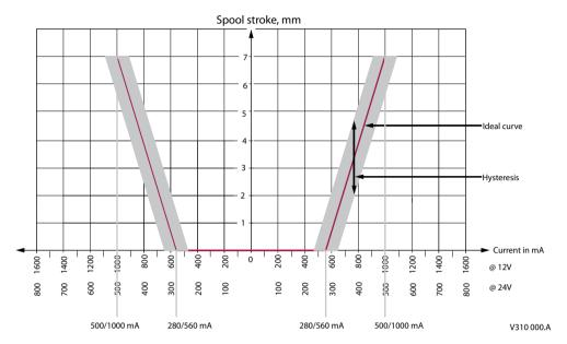
PVHC current response and hysteresis @ 25 bar  $P_p$ , 21 ctS, 25 °C. The ideal curve is determined by the main spool neutral spring. The PVHC has high hysteresis. The hysteresis is affected by viscosity, friction, flow forces, dither frequency and modulation frequency. The spool position will shift when conditions are changed e.g. temperature change.
