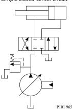
Once the closed center valve is opened, the PC control senses the immediate drop in system pressure and increases pump flow by increasing the swashplate angle.
