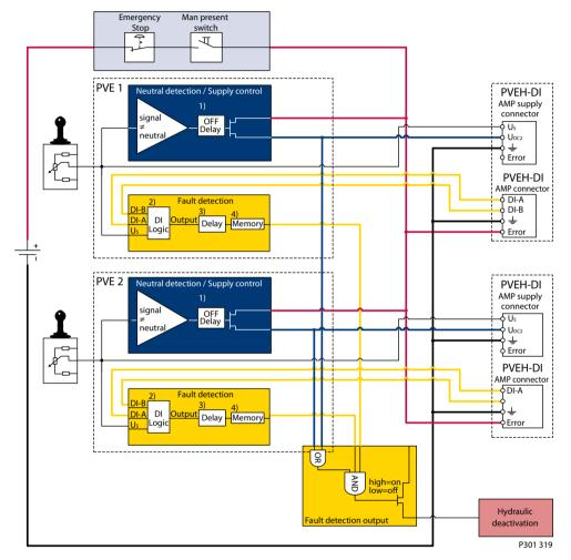
System Control Logic e.g. PLUS+1° for signal monitoring and triggering signal for deactivation of the hydraulic system.
