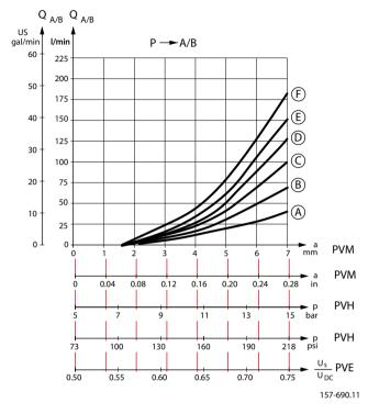
Set pressure difference between pump pressure and LS signal = 15 bar [218 psi] measured at the P-port of the valve.
