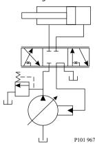
Most load sensing systems use parallel, closed center, control valves with special porting that allows the highest work function pressure (LS signal) to feed back to the LS control.
