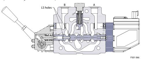
Option mounting is defined as installing the PVM on the "B" port side of the PVB. Because of this, the PVE or PV cover (PVH, PVMD, PVMR, PVMF or PVHC) would be on the "A" port side of the valve.
