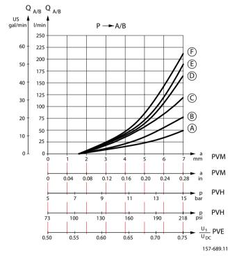
Set pressure difference between pump pressure and LS signal = 20 bar [290 psi] measured at the P-port of the valve.
