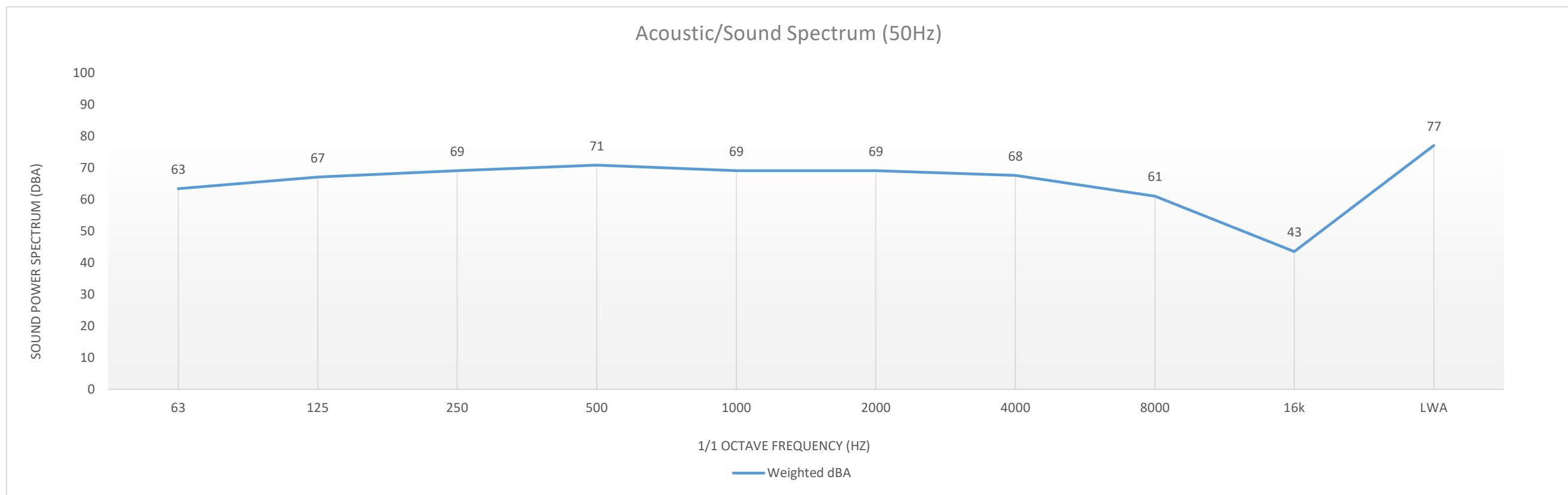
Acoustic spectrum data are calculated by addition of sound power levels of compressor and fan motor at full speed according to EN13215 conditions.
