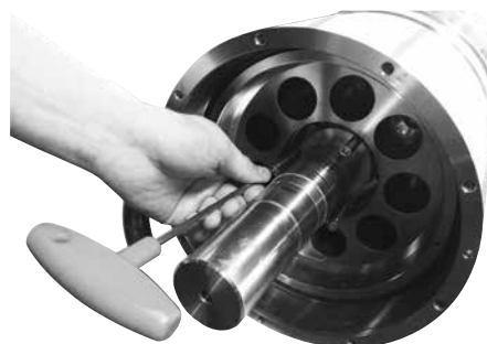
14. Unscrew the 3 valve plate fixtures, using a 8 mm Allen key.
