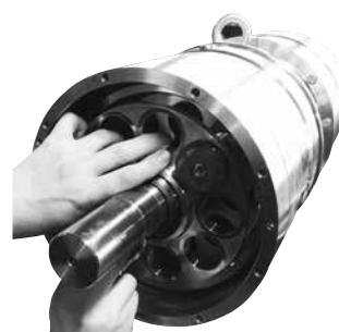
16. Spray clean filtered water over all the pistons and inside the cylinder barrel. Mount the retainer plate and while holding the retainer plate with one hand insert carefully two pistons to keep the retainer plate in place.
