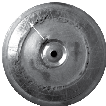
3. Picture 3: Cavitation of the piston shoes. All pistons must be replaced within the next 1000 hours.
