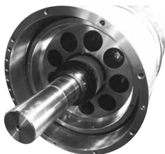
15. Spray the shaft with clean filtered water and mount the spring package, the distance washer and the retainer ball (with the spherical surface towards you) (if your pump is an APP / APP S / APP S 674 53 there is no distance washer in the pump).
