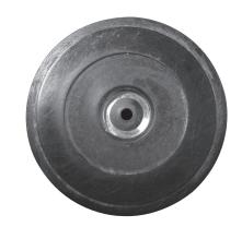
1. No wear or cavitation of the piston shoe. New inspection is required in 4,000 hours.
