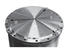
16. Place three bolts in mounting flange. Turn each bolt one round at a time to ensure mounting flange is mounted as straight downwards as possible. Be careful not to squeeze O-ring.
