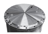
Unscrew the remaining three bolts. Turn each bolt one round at the time to make sure that the flange is removed as straight forward as possible.
