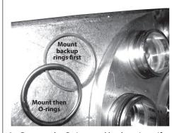
Remove the O-rings and backup rings. If they have been removed they can not be reused.
