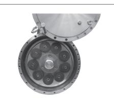
4. Place the retainer ring in an odd angle corresponding to the orientation of the swash plate.
