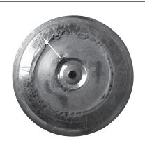
3. Cavitation of the piston shoes. All pistons must be replaced within the next 1,000 hours.
