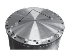
Place the swash plate upside down. Remove the 2 bolts holding the swash plate. Remove the mounting flange from the swash plate.
