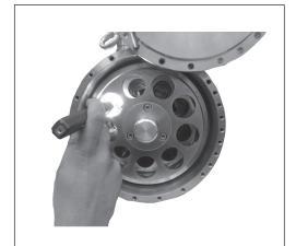
13. Inspect the piston liners. Replace any worn parts.
