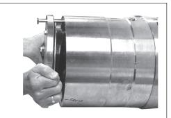
6. Remove the flange when the remaining three screws have been loosened. The guide bolt must remain mounted.
