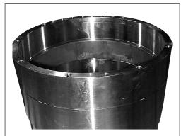
4. Position housing alingning pin hole over pin. Carefully press the port flange downwards. Do not squeeze the O-ring. If the O-ring is damaged, the pump will leak. Screw in at least two screws.
