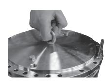
Screw the eye bolt in the M8 hole in the middle of the flange. Pull it straight upwards.
