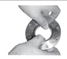
Remove ceramic ring from flange by gently pushing it from the back of the sealing ring.
