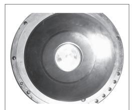
11. Swash plate must be placed so that its surface is not scratched. For further disassembling of swash plate, see page 10.
