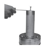
4. Remove the press bush again by screwing the nut counter-clockwise.
