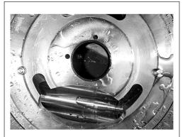
2. Place port flange with O-ring pointing upwards.
