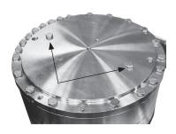
8. Using a 13 mm combination wrench, remove all the bolts on the mounting flange except the three shown in the next picture.
