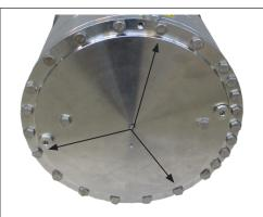
2. Loosen all screws on the pump except the three screws as shown in the picture above.
