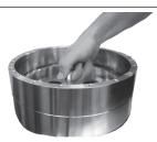
15. Mount a 8 mm eye bolt in the cylinder barrel. Pull straight upwards. A continuous lift will elevate the cylinder barrel out of housing. This can only be done if shaft seal is removed.
