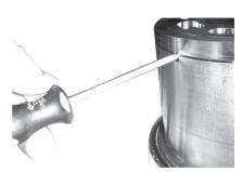
Push a screwdriver into the hole between cylinder barrel and valve plate. Carefully push downward the screwdriver so that it makes a gap between cylinder barrel and valve plate. Use this gap to put in another screwdriver and loosen the valve plate from the cylinder barrel.
