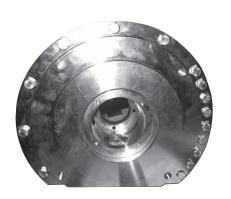
5. Place housing horizontally. Screw in the rest of the screws on port flange. Tighten screws to a torque of  $30 \pm 2$  Nm.
