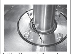
Using a 10 mm combination wrench, unscrew the four bolts from shaft seal flange.
