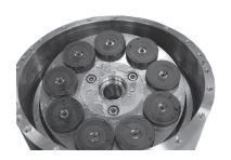
12. Remove by hand the pistons one by one. Be careful not to scratch the pistons. Tilt the retainer plate to horizontal position for easy removal of pistons, if required.
