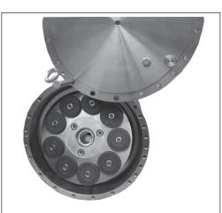
8. Adjust the retainer plate to be parallel to the end flange.
