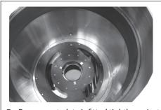
Ensure port plate is fitted tightly against the bottom.
