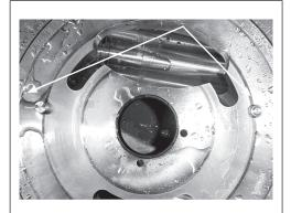
18. Remove, by hand, the two pins.
