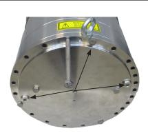
4. Unscrew the remaining three screws by using a combination wrench to turn each screw a couple of rounds at a time so the flange is removed as straight outward as possible.
