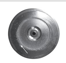
2. Cavitation of the piston shoes. New inspection is required in 2,000 hours.
