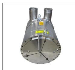
7. Mount the three screws as shown above. Tighten them to a torque of 30 Nm  $\pm$  3 Nm.
