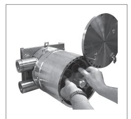
1. Carefully push the retainer ring in place.
