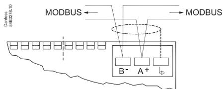
It is **important** that the installation of the data communication cable is performed correctly with sufficient distance to high voltage cables.
