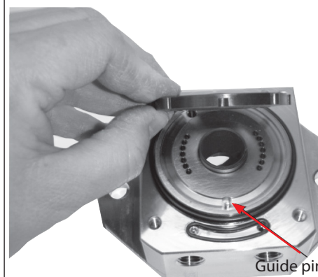
4. Mount port plate in its right position using pin as guide.
