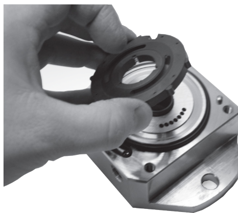
11. Remove port plate from flange.
