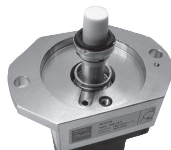
20. Wet shaft seal and mount/slide it over bush.
