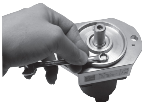
27. Tighten screws to a torque of 7 Nm.
