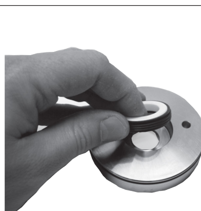
24. Wet shaft seal with water and mount it in front cover. .
