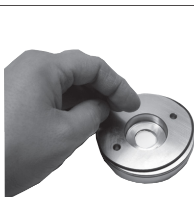
23. Mount O-ring on front cover.
