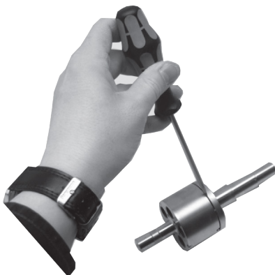
15. Loosen thrust plate using a screwdriver. Place screwdriver in slot of thrust plate.
