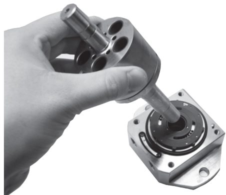
10. Remove cylinder barrel.
