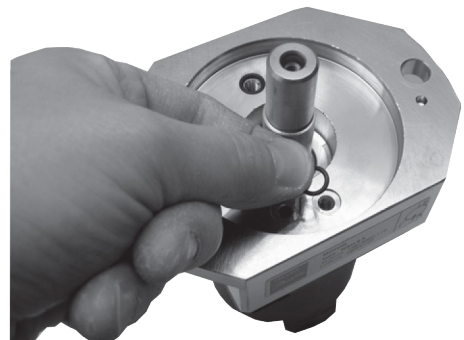
16. Mount the two O-rings in the flange.
