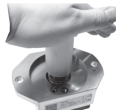
22. Press shaft seal in position.
