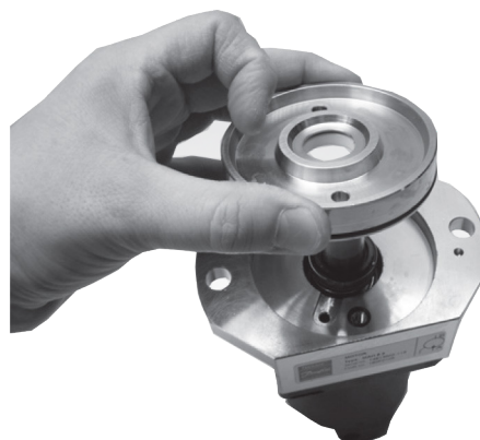
26. Mount front cover and align it to screw holes.
