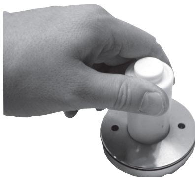
25. Press shaft seal into front cover using shaft seal tool. Ensure that it is pressed to the bottom.
