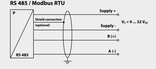
The Modbus protocol demands low process and RAM requirements on the receiver side. Data is transmitted in 8-bit bytes, one bit at a time, at baud rates ranging from 1,200 bits per second (baud) to 115,200 bits per second. Modbus RTU has excellent scalability as it can handle up to 247 nodes.
