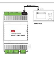
For cable <3 meter RJ CAN connector Termination Jumper between R and H For cable >3 meter (only EKE 1C and EKE 1D) 2-way screen connector for power supply 4-way screen connector for CANbus network
