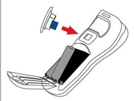
2. Place the EEPROM and the charged alkaline batteries.
