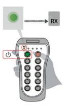
**4.** If the transmitter does not have the STOP button, press the start button. The status LED will blink in green until the transmitter is linked with the receiver.
