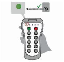
**5.** When the receiver confirms the link, the status LED will turn into fixed green, and will enter working mode. The system will be fully operational in order to action any maneuver.
