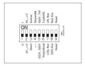
The actuator has a function selection DIP switch under the removable cover. In particular, if SW6 is set to ON, the actuator will perform as 3-point actuator.
