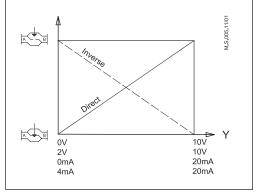
If set to OFF position, the actuator is working in sequential range 0(2)..5 (6)V or 0(4)..10 (12)mA. If set to ON position, the actuator is working in sequential range; 5(6)..10V or 10(12)..20mA.
