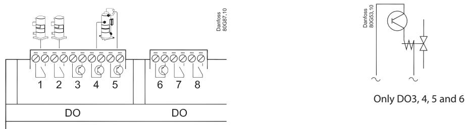
The capacity is divided into period times as "PWM per". 100% capacity is delivered when cooling takes place for the whole period. An off time is required by the bypass valve within the period and an on time is also permitted. There is "no cooling" when the valve is on.
