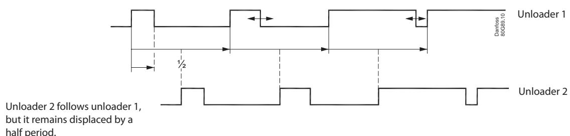
CRII 6: The pulse signal can also be used to control one CRII with three unloaders (6-cylinder version).
